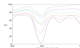
ATR FTIR spectra of polymers DMVP:TPGDA. Dependence of intensity of P-O-C stretching band on DMVP molar ratio in copolymer.
