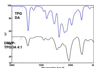
FTIR ATR spectra of TPGDA and copolymer DMVP-TPGDA 4:1
