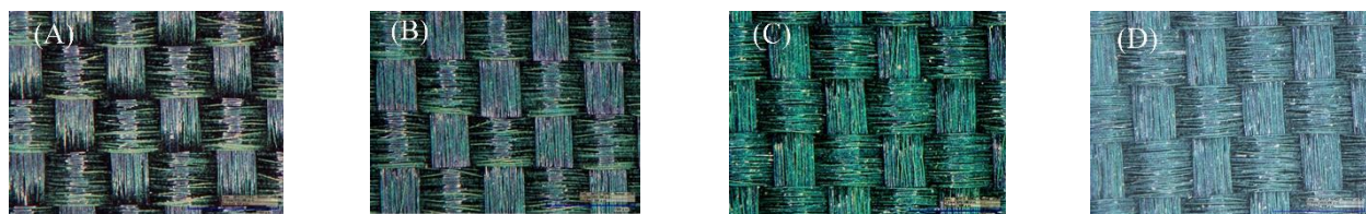
Figure 3. The structural color of fabrics with different \text{Cu}_2\text{O} microsphere concentration (a) 0.5 wt.%; (b) 1.0 wt.%; (c) 3.0 wt.%; (d) 5.0 wt.%
